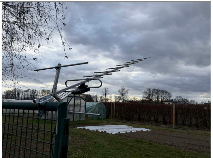
Figure 19 – ATK-10 directional antenna
